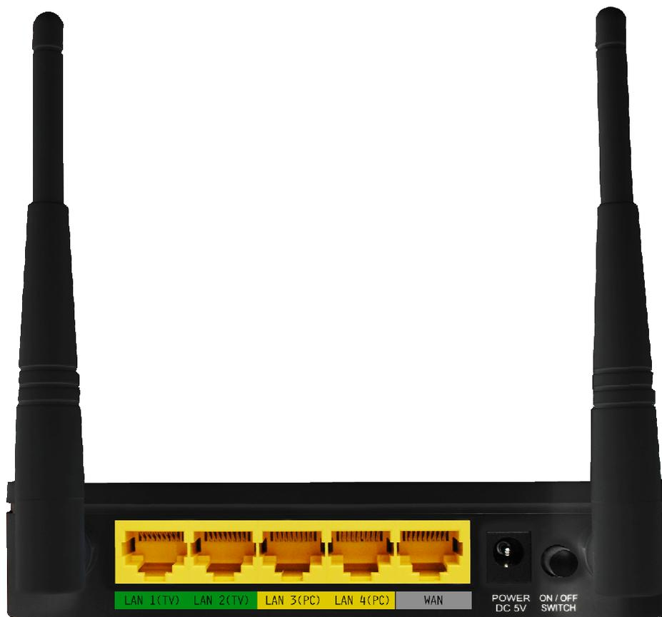
*Figure 2: Rear Panel Connections*
